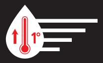
A BTU, or British Thermal Unit, is the amount of energy needed to heat one pound of water by one degree Fahrenheit.
