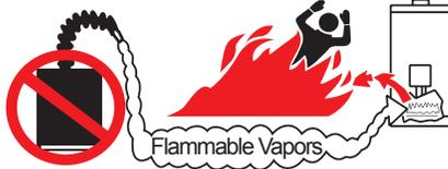
Do not install water heater where flammable products will be stored or used unless the main burner is at least 18" above the floor. This will reduce, but not eliminate the risk of vapors being ignited by the main burner.
