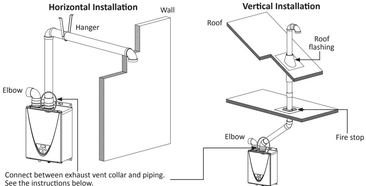
Connect between exhaust vent collar and piping. See the instructions below.
