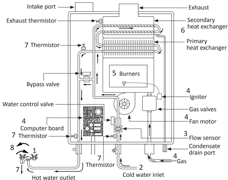
\*This diagram illustrates tankless water heater design concepts only and does not accurately represent the water heater's physical description.
