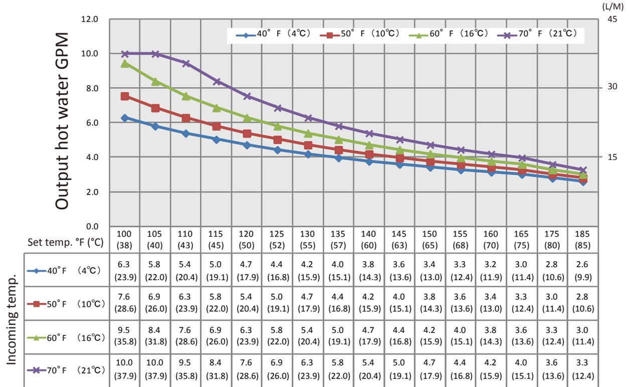
When the set temperature is 130 °F (55 °C) or higher, maximum flow rate is limited to 8.0 GPM (30.3 l/m).
