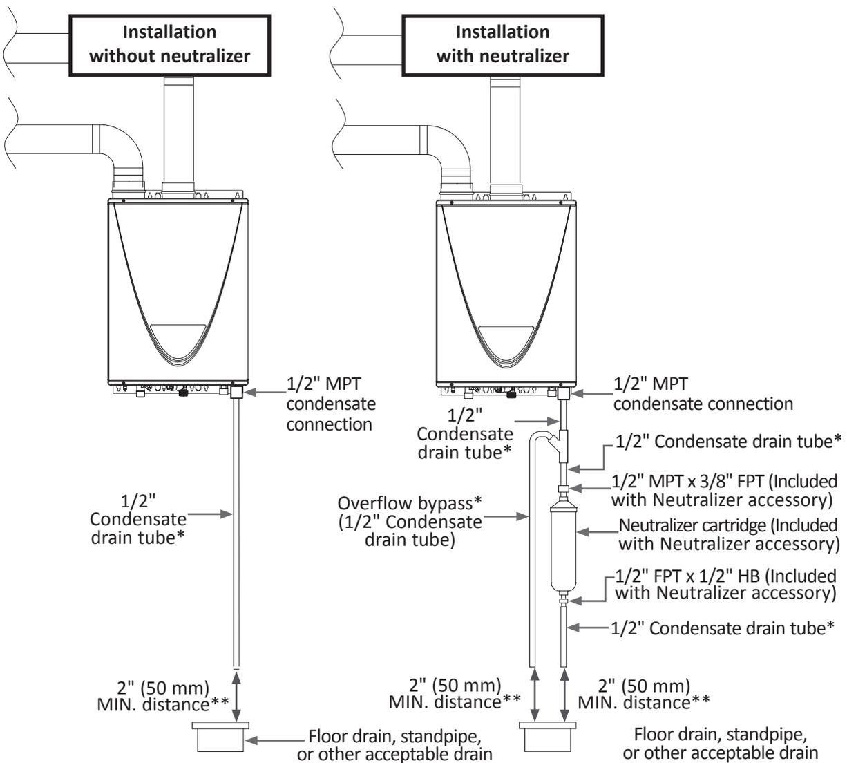
\*Maintain downward slope, including installations in which the drain is not directly below the heater.
