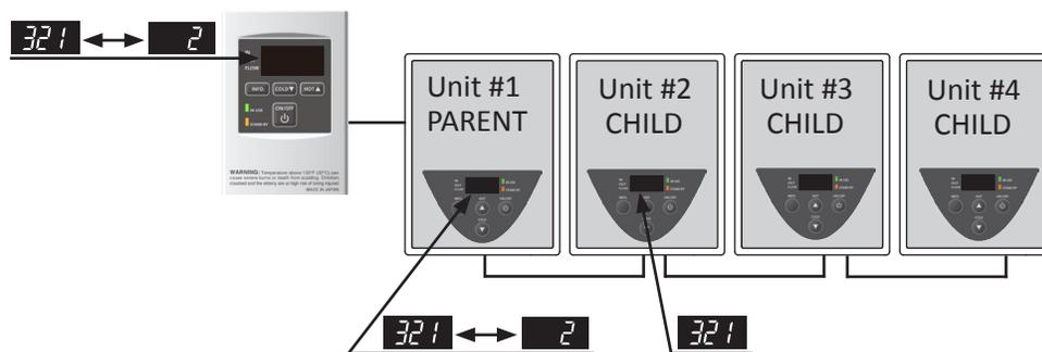
Unit #2: "321" will flash intermittently on the display. The green LED on the computer board will flash twice, just like in the single unit example.
