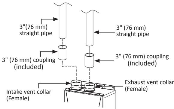
1. Connect 3" (76 mm) couplings directly on the exhaust and intake vent collar of the water heater.
