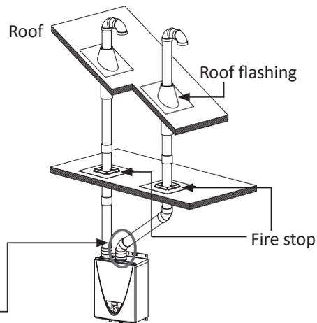
Connect between exhaust vent collar and piping.
