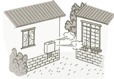
Do not install this water heater under an overhang less than 3 ft (914 mm) from its top or eaves. The area under an overhang must be open to three sides (Outdoor model only).
