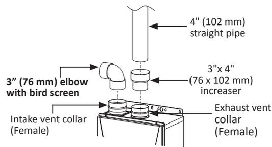
1. Connect a 3" (76 mm) elbow directly on the intake vent collar of the water heater.
