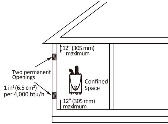
Figure 2 - Direct to outdoors openings
