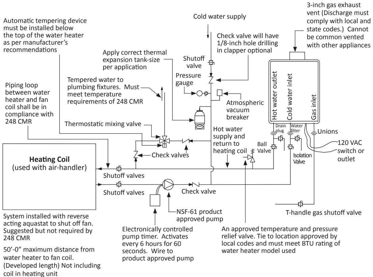
*The recirculation pump is to provide no less than 2 GPM (7.5 L/min) and no more than 4 GPM (15 L/min) through each activated unit in the system*
