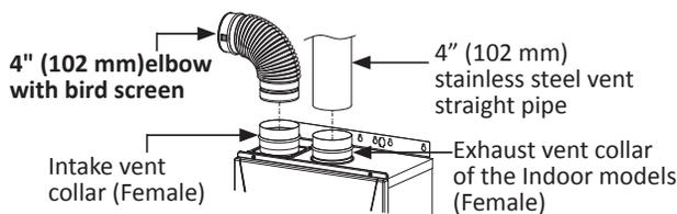
1. Connect a 4" (102 mm) stainless steel vent straight pipes directly on the exhaust vent collar of the water heater.
