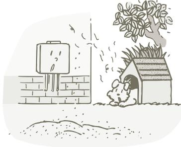
Do not have the vent terminal pointing toward any opening into a building. Do not locate your heater in a pit or location where gas and water can accumulate.
