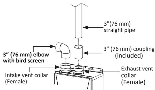
1. Connect a 3" (76 mm) elbow directly on the intake vent collar of the water heater.
