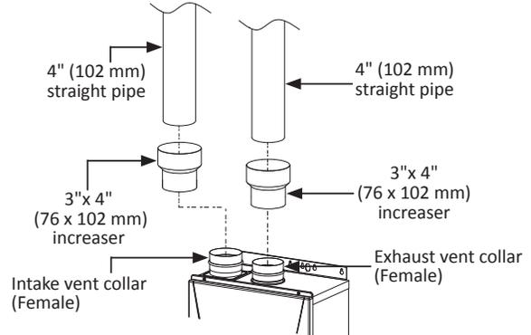
1. Connect 3"x 4" (76 x 102 mm) increasers directly on the exhaust and intake vent collar of the water heater.
