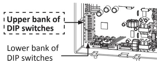
Set DIP switches shown in the table below depending on the vent diameter and length.
