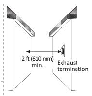
Exhaust and/or direct vent sidewall terminations should be at least 2 ft (610 mm) away from an opposite surface/wall. Do not place the termination directly in front of an opening into a building.
