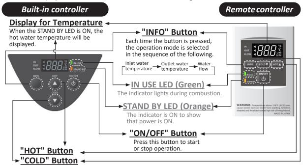
Press the "HOT" button or the "COLD" button to adjust the hot water temperature.
