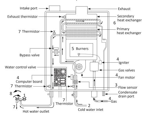
\*This diagram illustrates tankless water heater design concepts only and does not accurately represent the water heater's physical description.
