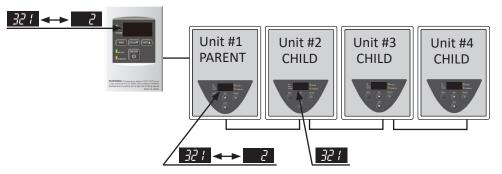
Unit #2: "321" will flash intermittently on the display. The green LED on the computer board will flash twice, just like in the single unit example.
