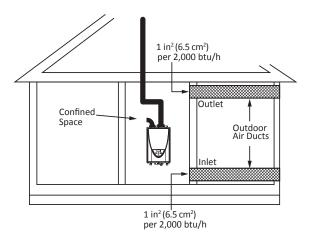
Figure 4 - Horizontal duct openings
