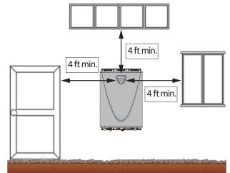
Locate the outdoor water heater so it's vent terminal meets the following clearances. Locate the vent terminal of an indoor heater to meet the following clearances:
