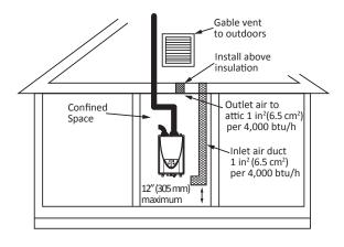
Figure 3 - Vertical duct openings
