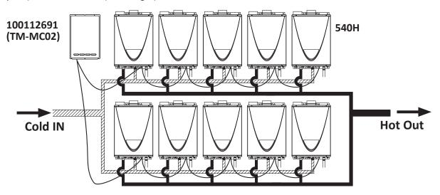
An individual cut-off switch is recommended for each unit in a Multi-Unit System for the purpose of maintenance.
