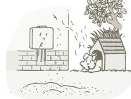
Do not have the vent terminal pointing toward any opening into a building. Do not locate your heater in a pit or location where gas and water can accumulate.
