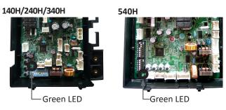
Error code on the computer board Indicated by 1/2-second flashes on the Green LED.
