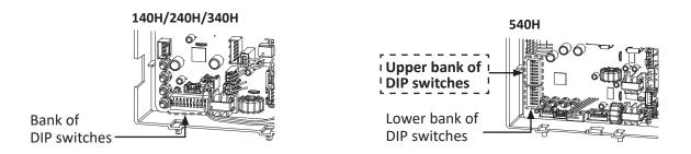
Set DIP switches shown in the table below depending on the vent diameter, the installation, and the vent length.
